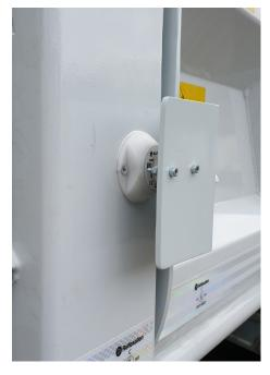
From a technical point of view, the solution for detecting the opening of the sides of hydraulic dump trucks is based on **an extremely light infrastructure** made up of magnetic sensors and magnets associated with Electro Maintenance's ATLAS Connect box.
